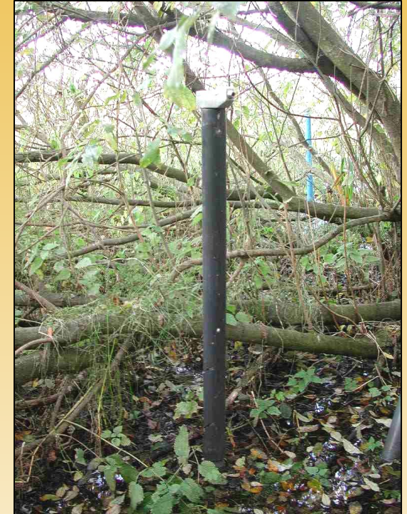
Groundwater dip well
