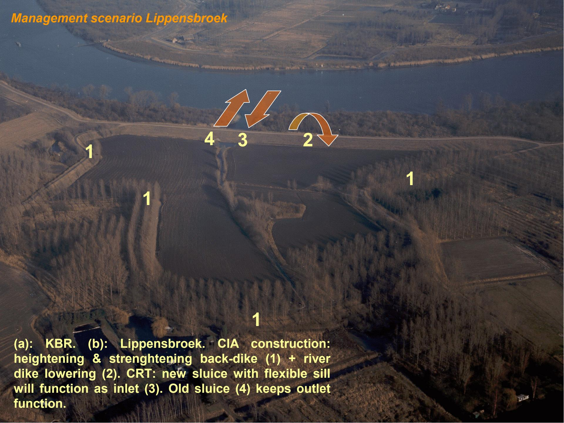
(a): KBR. (b): Lippensbroek. CIA construction: heightening & strengthening back-dike (1) + river dike lowering (2). CRT: new sluice with flexible sill will function as inlet (3). Old sluice (4) keeps outlet function.
